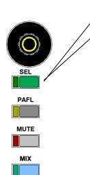
**Note:** For access to the channel processing using the SEL keys make sure the TouchScreen is not in SURFACE, MIXRACK or NAME&COLOUR mode.
